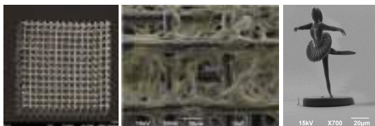
Fig. 1: (a) A spiral photonic crystal. (b) Scaffold for cell growth (c) A micro-dancer
